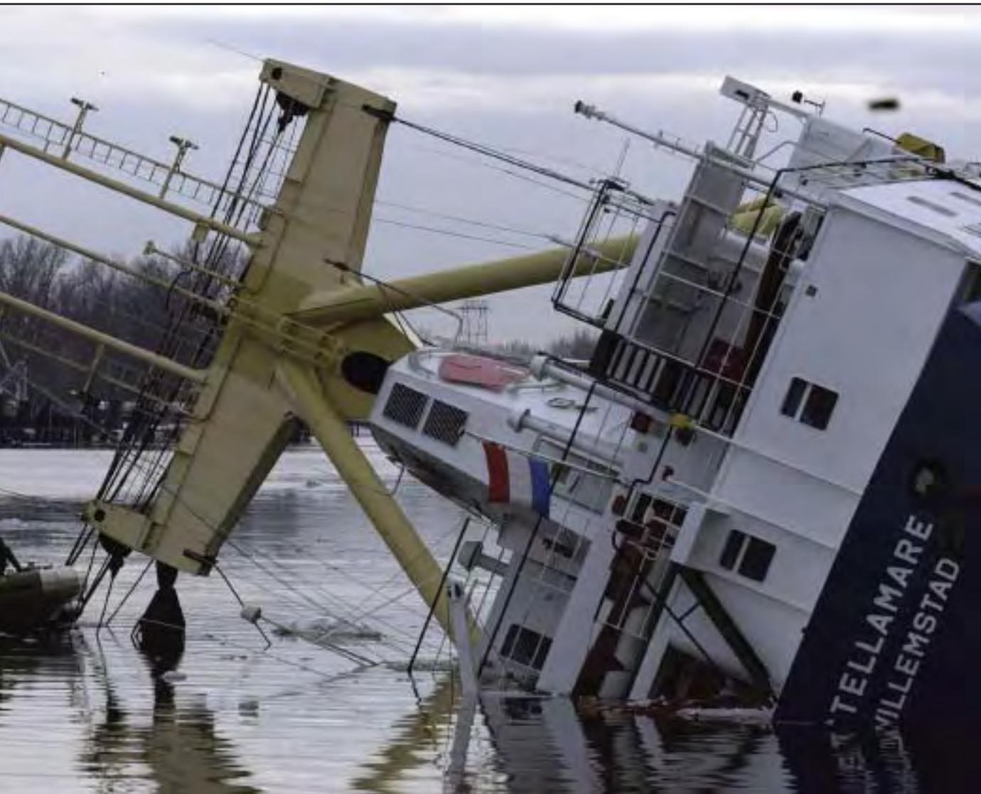
load. Here, the ballast water is referred to as “swing ballast” because its primary purpose is to help swing the load aboard. The applied ballast also has a tendency to lower the center of gravity a foot or two, but that helps to balance out the suspended load, which has a tendency to raise the center of gravity a few feet.
